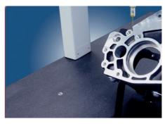
One-piece granite worktable provides a solid, stable work surface. The table is provided with M8 threaded inserts for part fastening.
